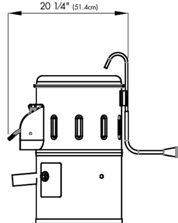
**Capacity:** Up to 20 lb (9kg) of potatoes per batch. Maximum capacity can vary based on size and shape of potatoes
